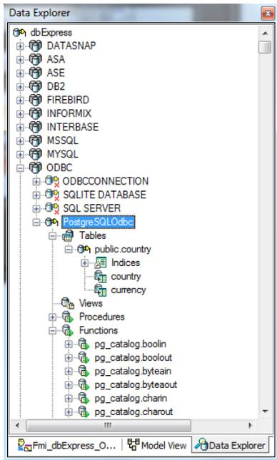
Figure 41. Data Explorer connected to PostgreSQL via dbExpress ODBC driver
