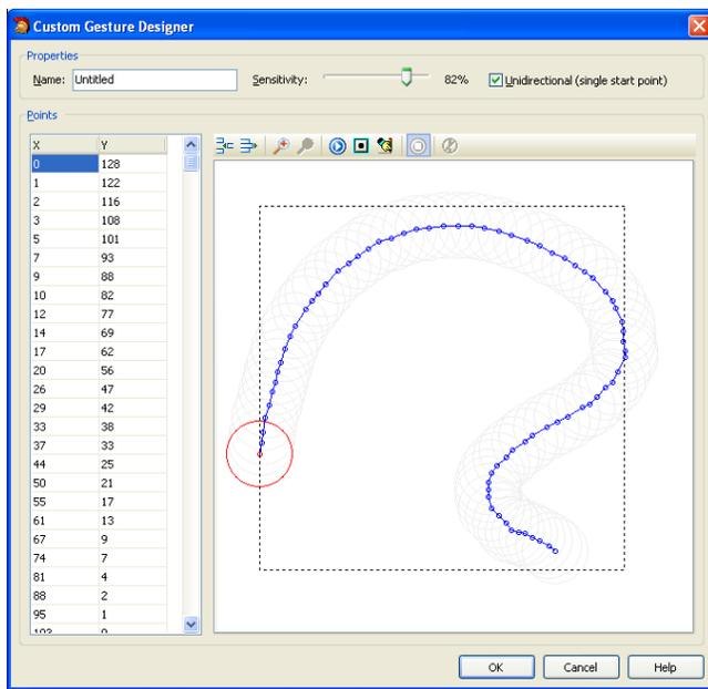
Figure 26. The Gesture Designer, allow developers to create and test gesture
